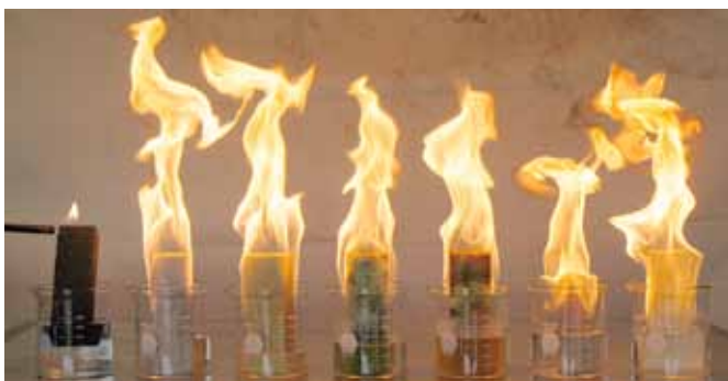
Undeniable proof of fire safety in the wicking test. Flammable liquids wick through and soak insulation materials
