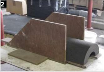
Use a mitre box to facilitate the cutting process of the FOAMGLAS<sup>®</sup> insulation. A mitre box consists of a 45° and 90° angle to assist with straight and diagonal cuts.
