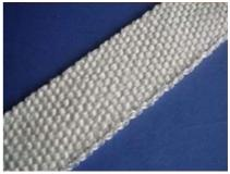
**ST 550 P** – The webbing type with plain weave and high tensile strength, made of pure texturized glass yarn. This is basic glass tape for general heat insulation and for reinforcing and coating other soft insulations. The tape is available with additional feature as coating reflective alufoil, red silicon elastomer also with metal wire reinforcement.
