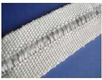
**ST 550 L** – The ladder tape woven with wrap yarns missing in the centre, the gap is around 25% of the tape wide. This tape is designed for sealing gases on flange with bolts and it gives easier installation and does securing fasteners in bolt line.
